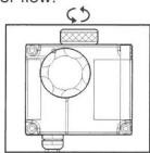
2. Unscrew Cell Cap, MCU or Autoclean.
