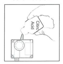
Ensure that the valves remain closed. Mix some Citric Acid with 15 ml water. Fill the Sample Glass Tube with the Citric Acid liquid and let it soak over night. Flush with clean water without gas.
