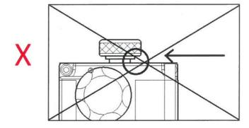
2. A not completely screwed down Cell Cap may allow formation of air bubbles and may influence with flow rate settings.
